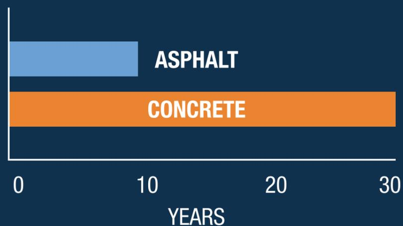
Concrete roads can be designed for 50 years or more, and they last around three times longer than asphalt roads before a first major rehabilitation is required.
