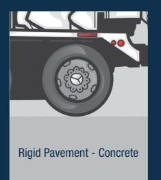
The deflection-induced fuel consumption on asphalt is more than twice as high as that on concrete of same thickness.
