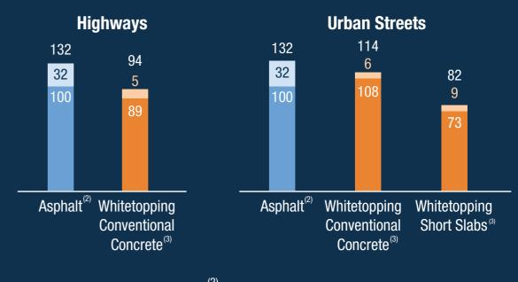
With solutions such as whitetopping, short slabs, and cement treated base concrete beats asphalt even on initial construction costs.
